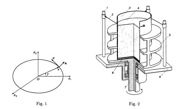
coaxiality of the stress and strain tensors were studied using a special stress gauge [16], which was placed inside the sample at a certain fixed depth. A vertical spoke was tightly fastened to the gauge to control the orientation of the gauge with respect to the axes of the elliptic holes of the loading plates. A flag whose plane coincided with the plane of the gauge was fixed at the free end of the spoke above the surface of the sample.
